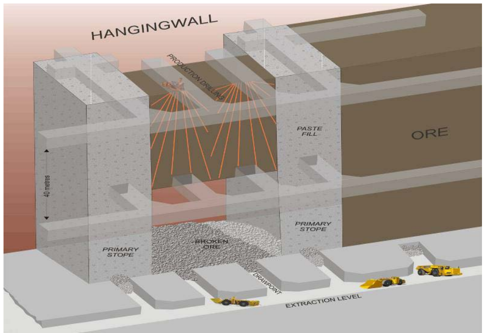
Figure 5: Long hole open stoping method (OZ Minerals, 2014)
