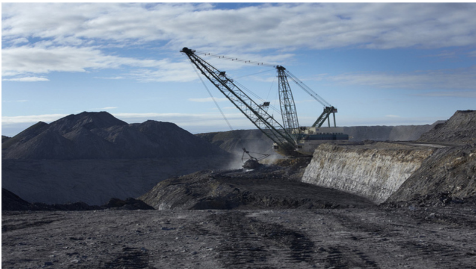
Figure 2: A dragline is removing overburden at Mount Thorley Warkworth (Chakraborty, 2017)
