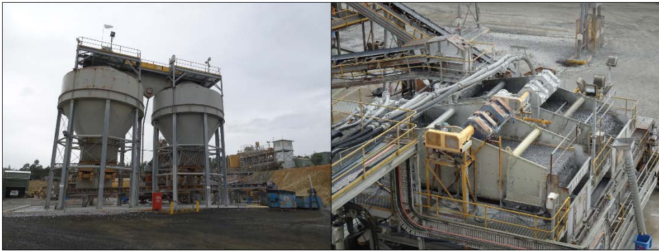
Figure 4: Impact mills/ centrifugal mills(left) and Classification (right)
