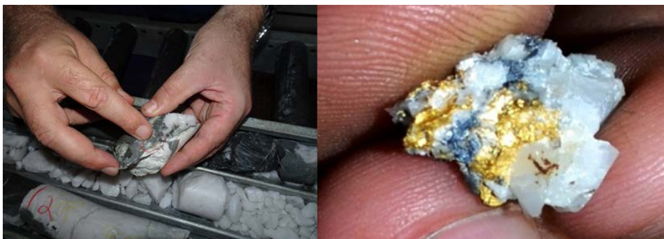
Figure 1: Left: A drukk core with gold content; right: Quarz rock with gold content
