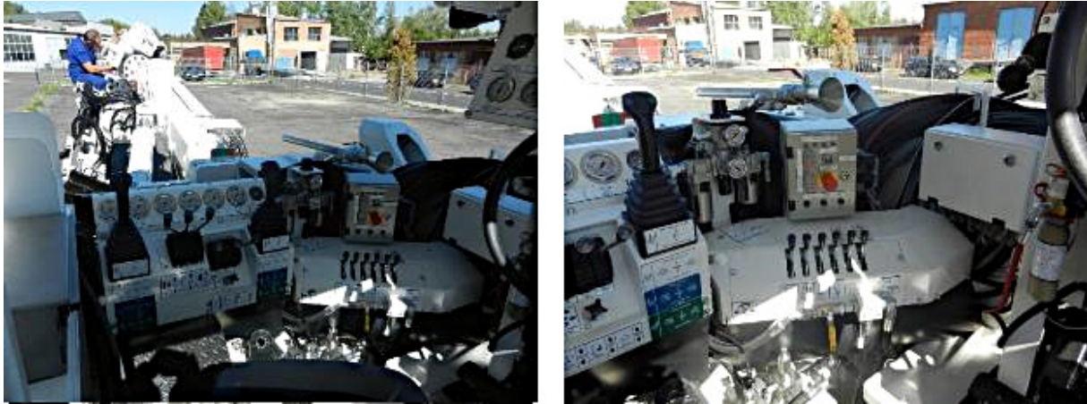
Figure 13: View from operator's compartment towards bolting mast. Source: Mine Master
