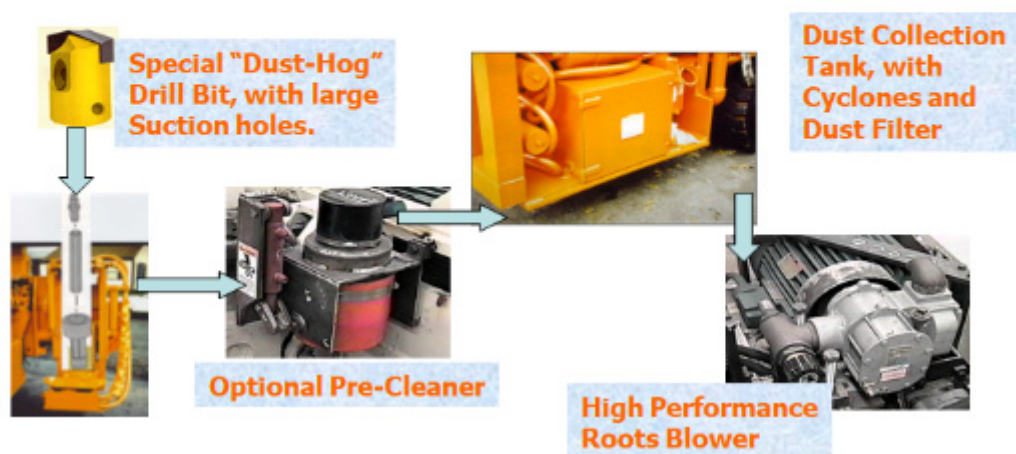
Figure 7: Diagram of dry drilling with dust collection.
