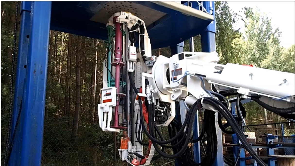
Figure 10: View of remote operated bolting mast under test bench. Source: Mine Master
